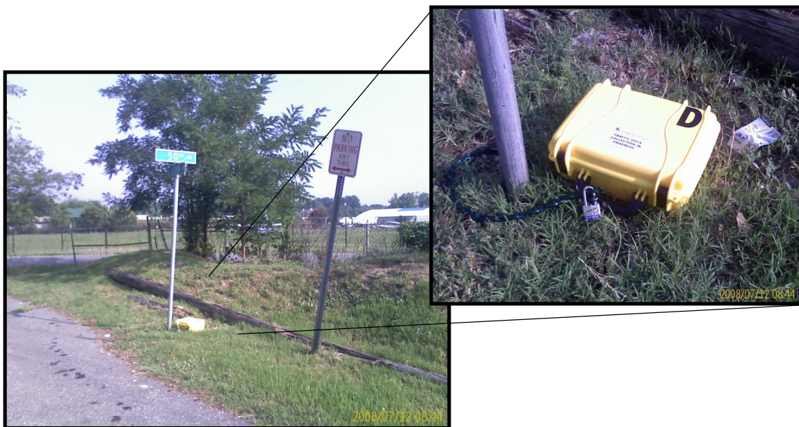
Figure 2 The Bluetooth detector is shown as it would be deployed during data collection. The unit sits on the ground and is tethered to an existing post.
